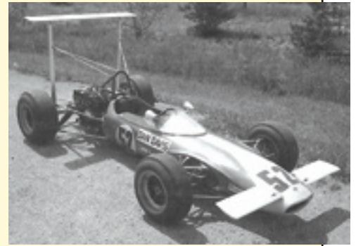
The Lotus 41C of Dan Davis in 1969 trim with suspension mounted high wing.
